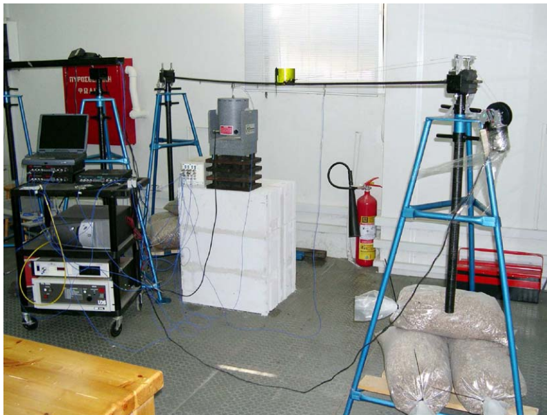
Fig. 2. The laboratory TV structure. A bridge with heavy vehicle type structure consisting of a steel beam, clamped close to its both ends on vertical stands, and a cylindrical mass sliding on it at a selected speed: (a) schematic diagram and (b) photo of the experimental setup [11].
